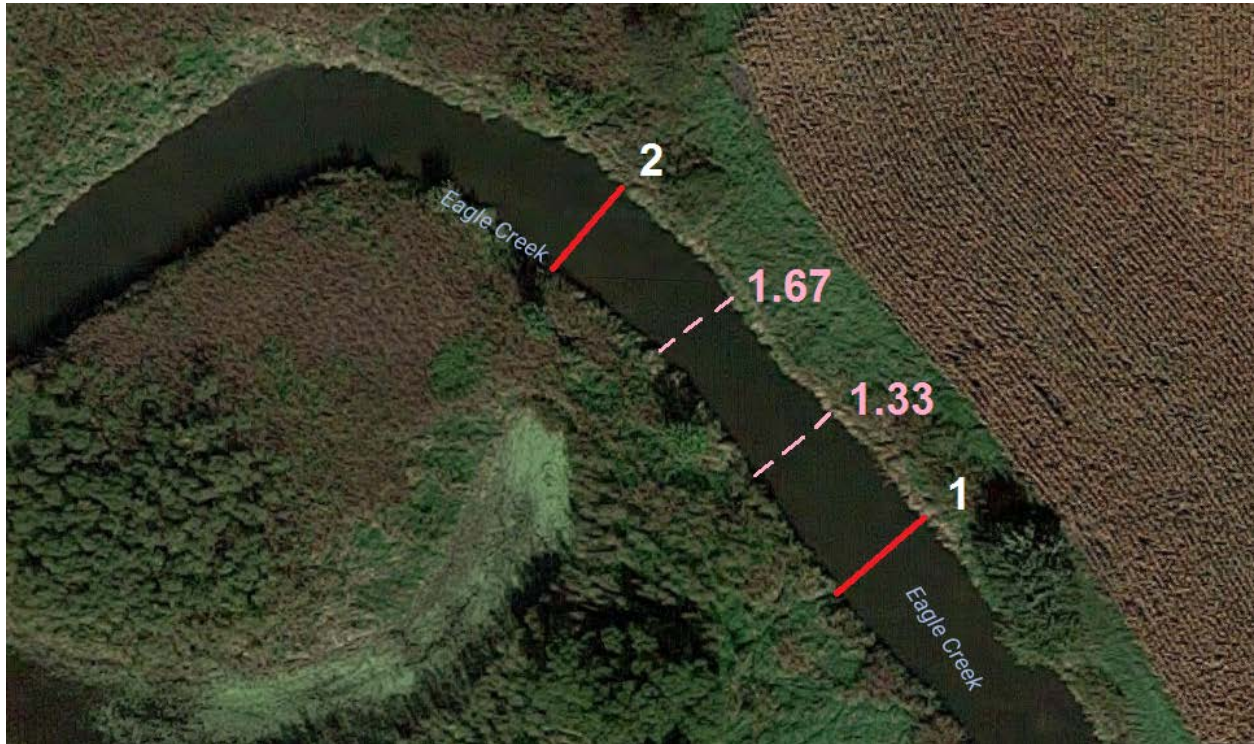
Figure 1G. Macrohabitat type, thalweg depth, and presence of soft/small sediment were recorded at each mini-transect line (pink dashed line) and each transect line (red line).
